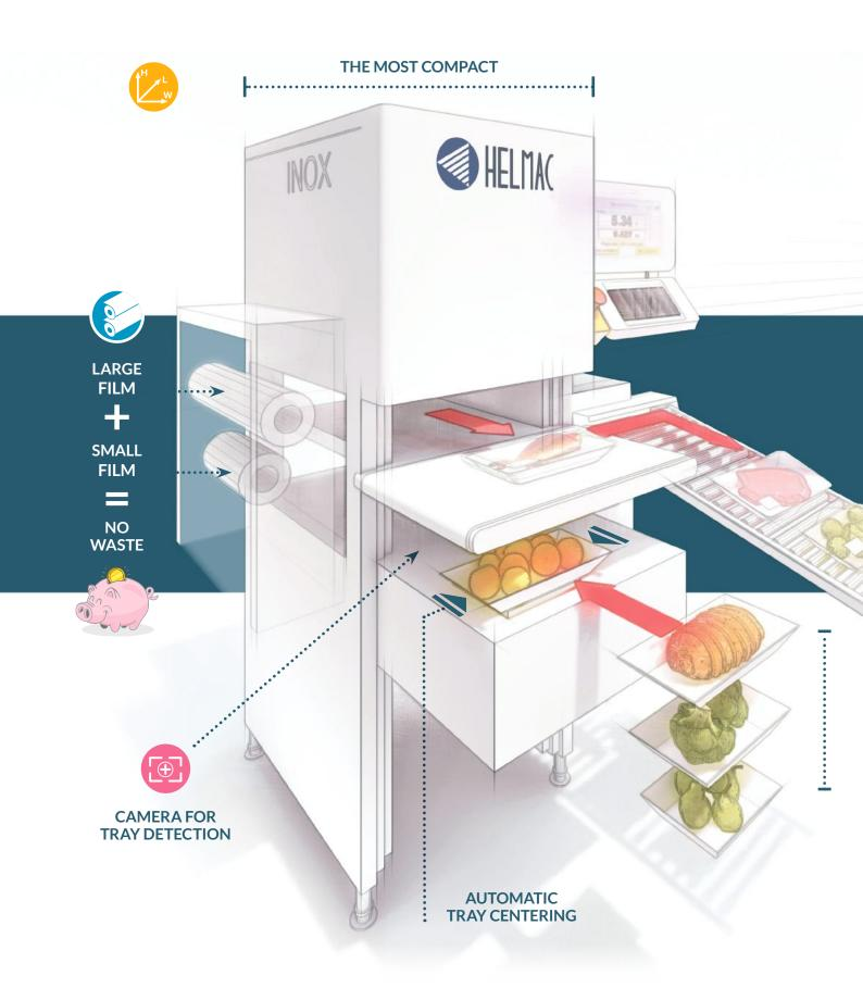
Automatic wrapping machine in stainless steel that **weighs, wraps and labels** up to 35 trays per minute, particularly suitable for deli, meat and produce department.
